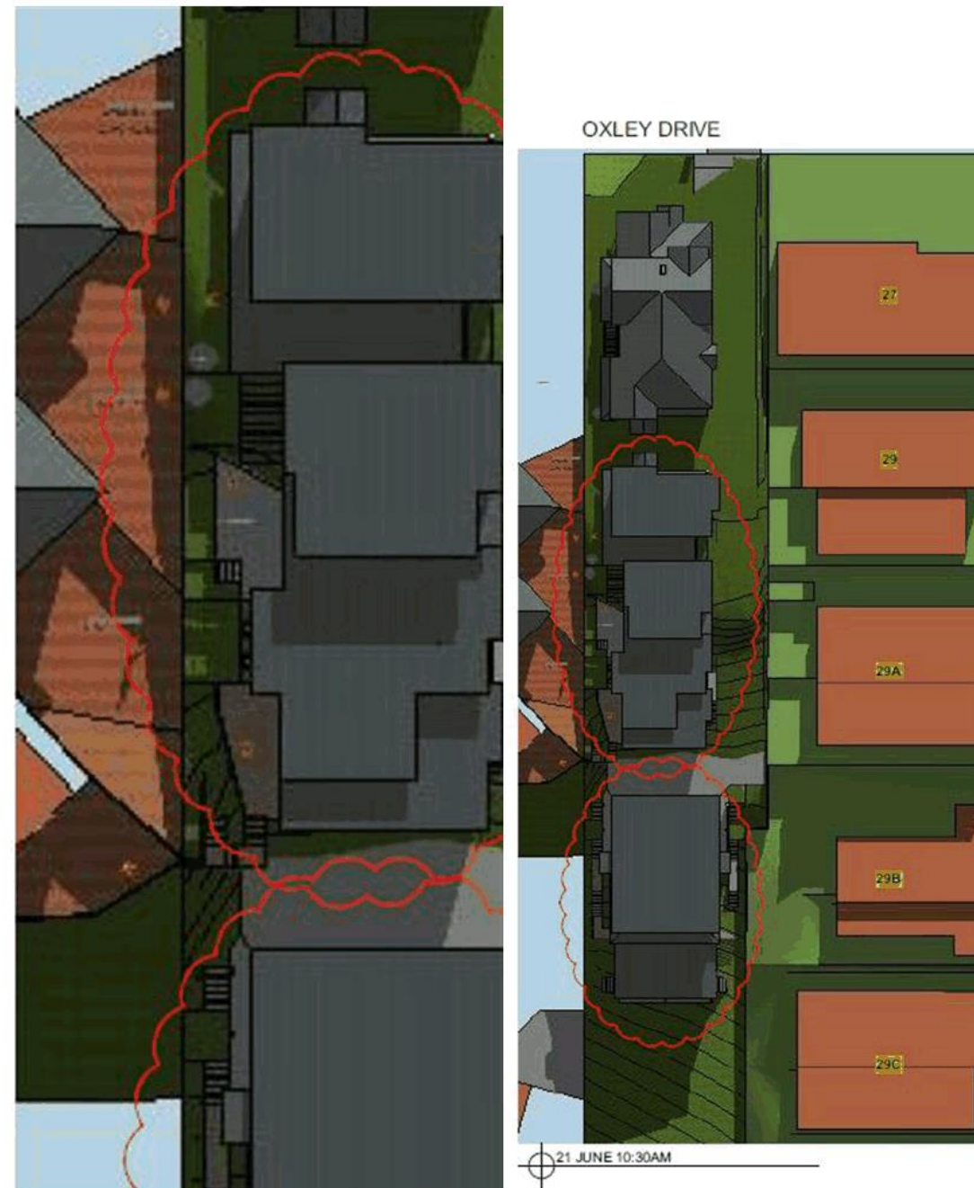
10:30am 21 June – Overshadowing of adjoining western units 3/23, 4/23, 5/23 and 6/23 private open space areas
