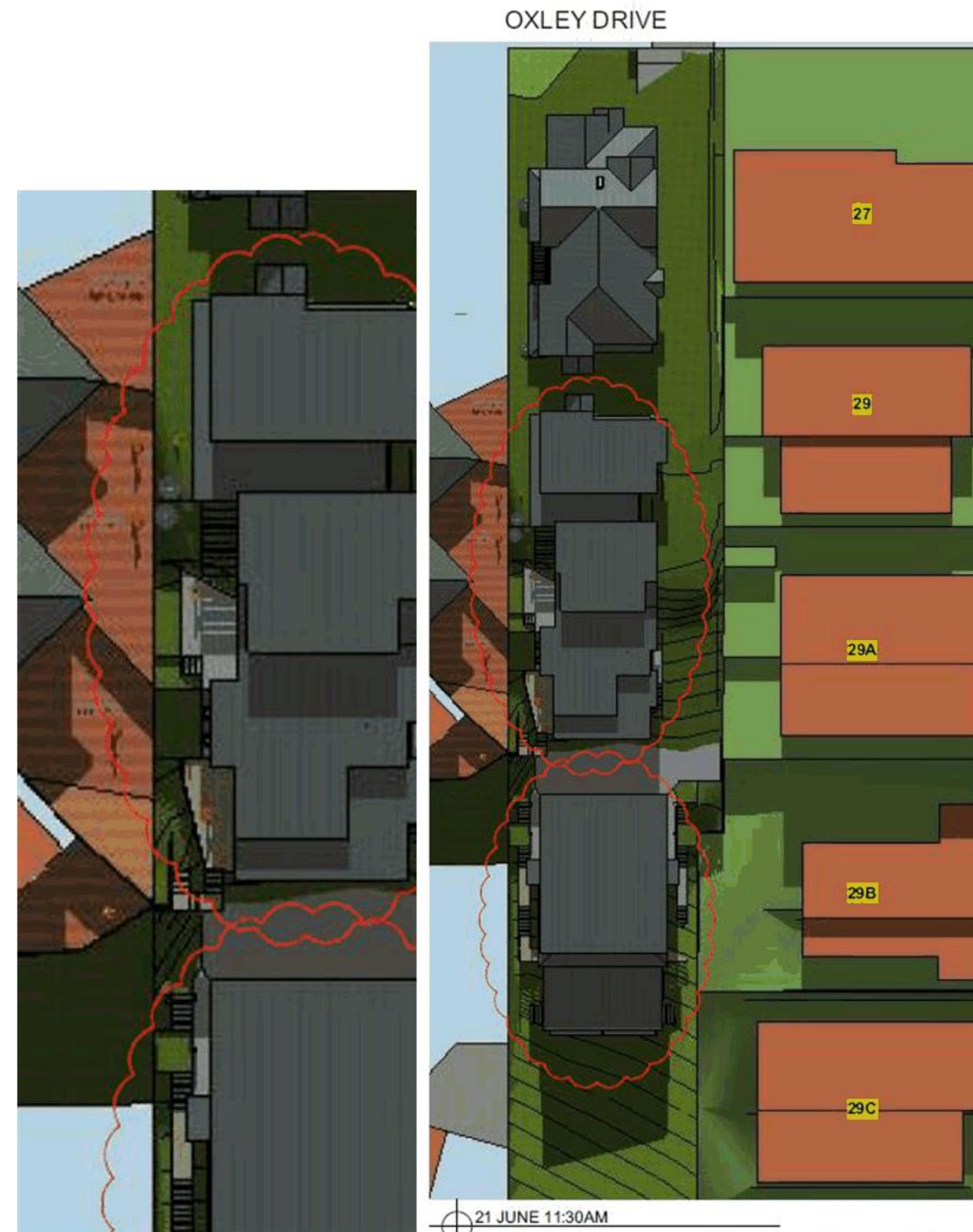
11:30am 21 June – Proposed development does not overshadow adjoining western units 3/23, 4/23, 5/23 and 6/23 private open space areas Proposed development does not overshadow adjoining eastern properties. Overshadowing largely contained within subject property.
