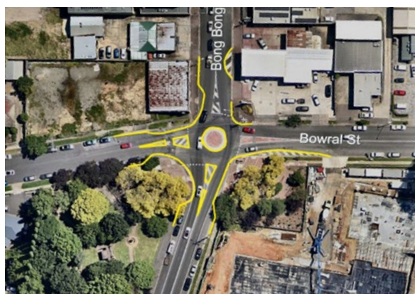
Figure 45 Improved pedestrian crossing treatment at the intersection of Bong Bong St and Bowral St
