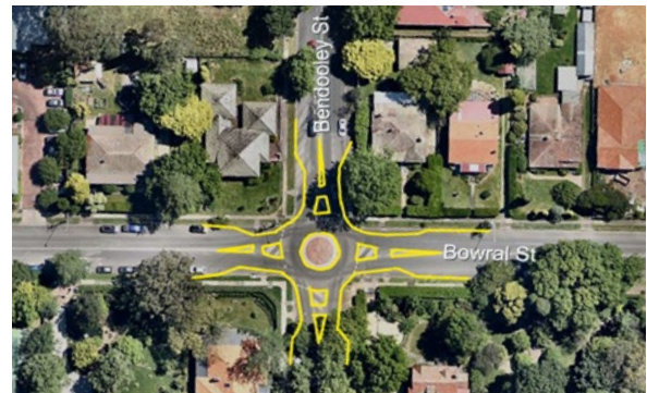
Figure 47 Improved pedestrian crossing treatment at the intersection of Bowral St and Bendooley St
