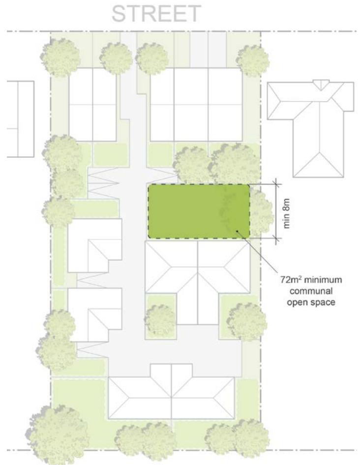
Figure 56 Communal open space should be provided where more than 10 dwellings are proposed
