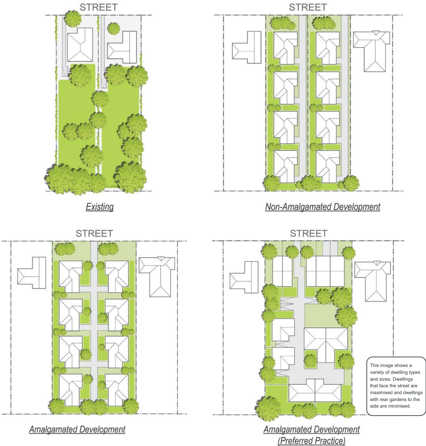
Figure 41 Amalgamating sites can reduce the amount of driveways required and increase the potential area for landscaping.
