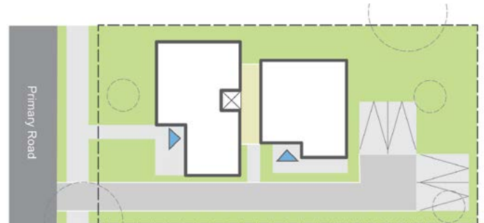
Manor House development with a single frontage to the street and on grade car parking to the rear
