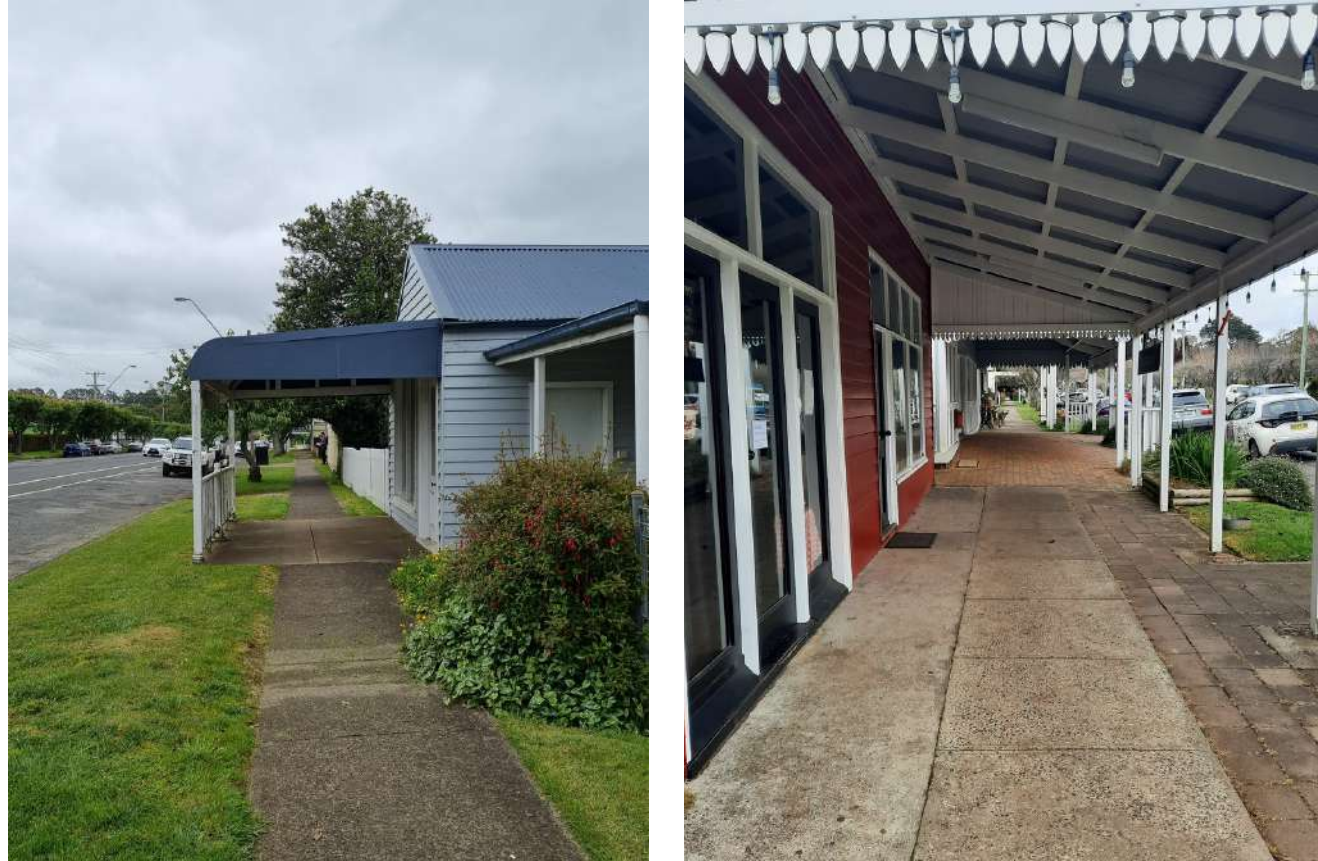
Example of Zero Lot Line in Robertson where buildings are located along the front boundary line.
