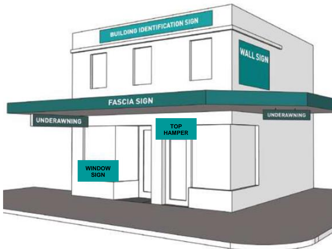
Figure A4.1.1 Typical Business Identification Signage on or Attached to a Building
