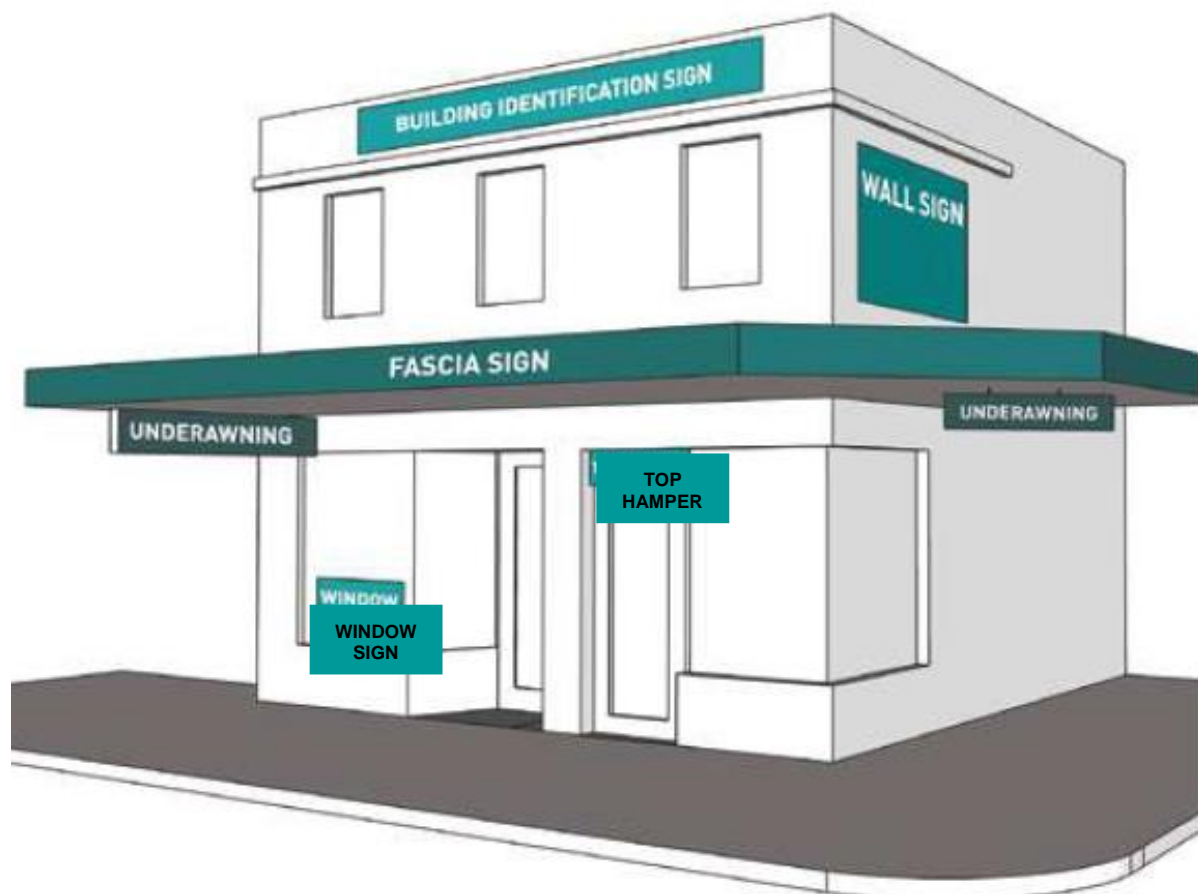
Figure A10.1.1 Typical Business Identification Signage on or Attached to a Building
