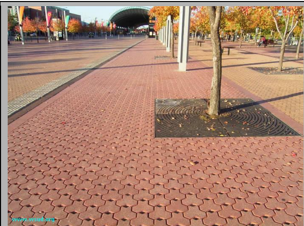
Photo*: Porous pavements and permeable street tree plantings located at Sydney Olympic Park, New South Wales.
